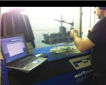
lift, airflow and velocity readings are taken. The same operation is also undertaken to the exhaust ports - the only difference being that the flow-bench is set to blow instead of suck, in order to simulate the pushing action of the piston as opposed to the sucking on the inlet side. With airflow readings taken, the ports can be modified and then re-tested to ensure the desired results are achieved.
